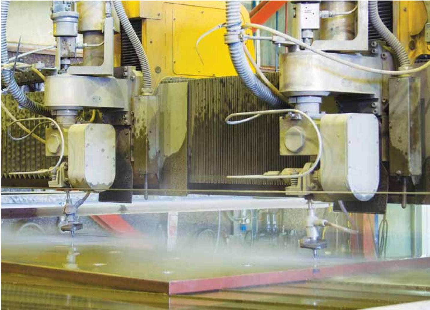
Waterjet cutting is used to cut the Hardox wear plate.
