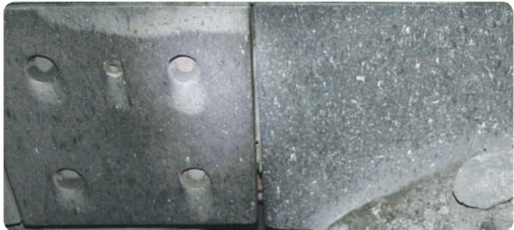
On the traditional plate, pictured left, crater wear is visible around the screw holes. The Hardox WRC plate to the right is mounted with our WRC screw with a conical head and in this plate it is almost impossible to discern the screws.
